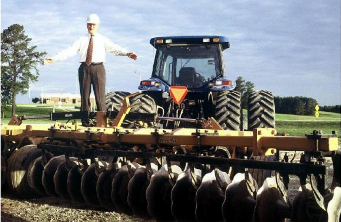
**24-inch diameter agricultural disk is used to break up compacted soils at the surface.**
