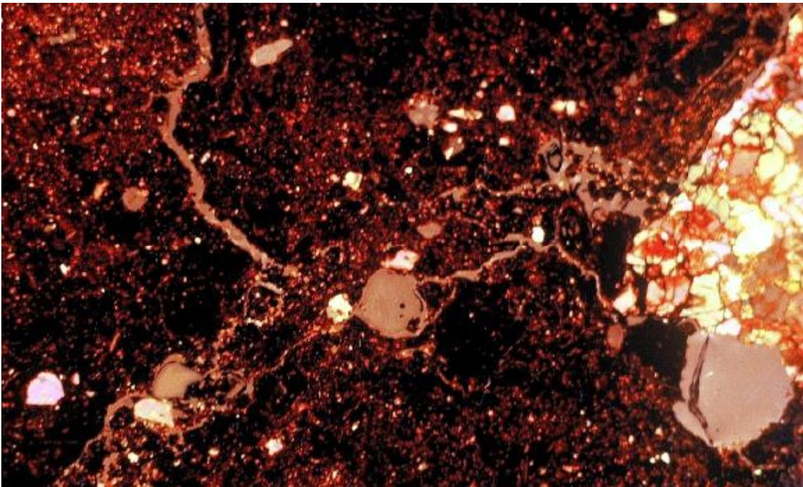
**Enlarged microscopic view of Cecil clay subsoil at forested site shows cross section of two tubular macro pores which receive water from topsoil reservoir (light gray areas are pores; the photograph also shows a large multi-colored sand grain).**
