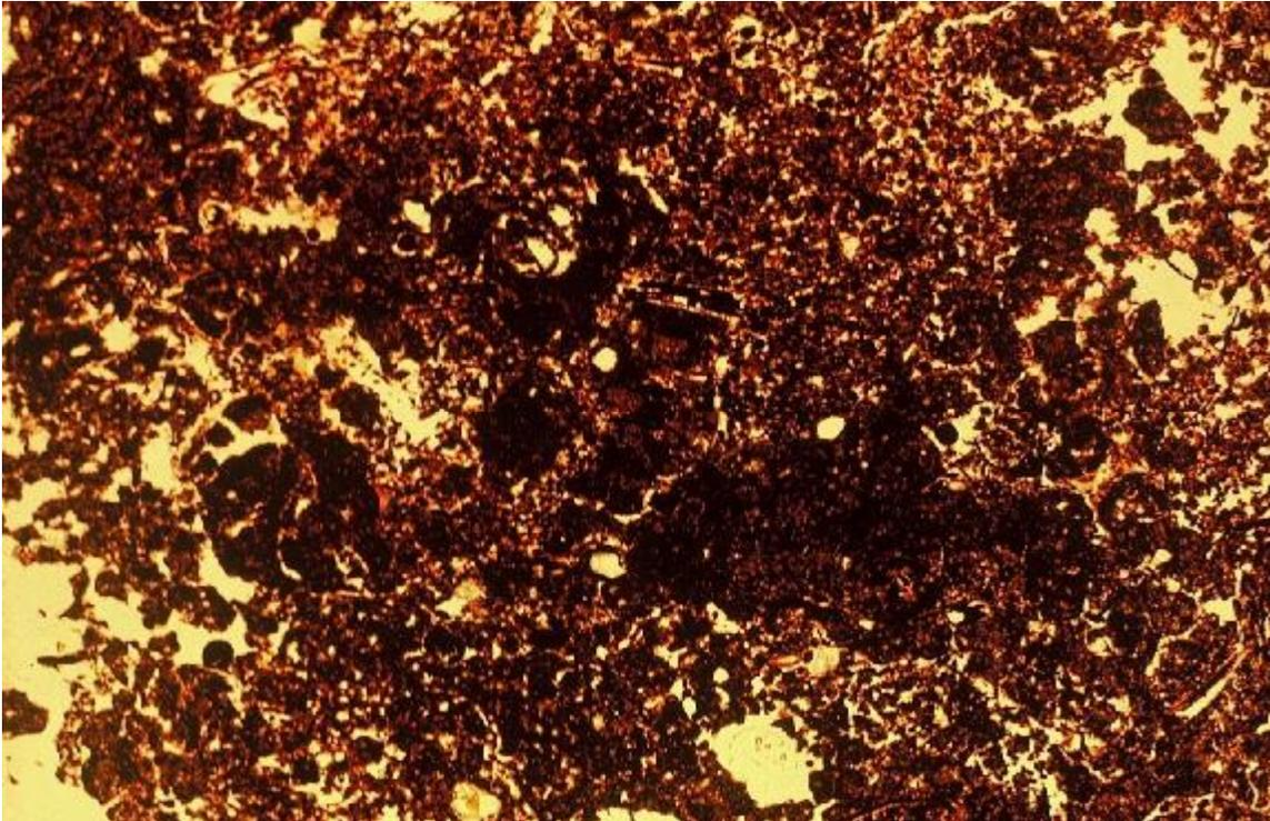
**Cecil sandy loam topsoil at forested site is very loose and porous (light areas are pores). Rainfall ponds in the topsoil reservoir prior to flowing into the subsoil.**
