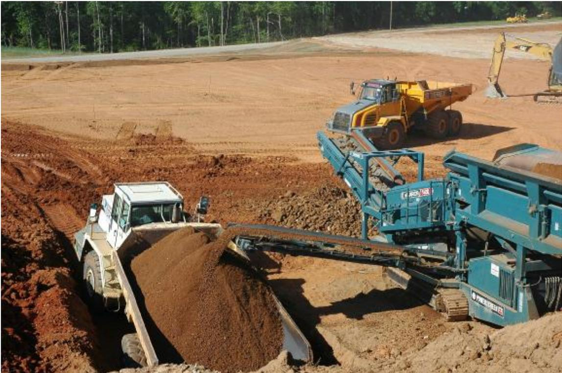
**Warrior 1400 power screener and loader is used for custom processing and blending of on-site soil materials, thus reducing or eliminating the need for importing topsoil.**
