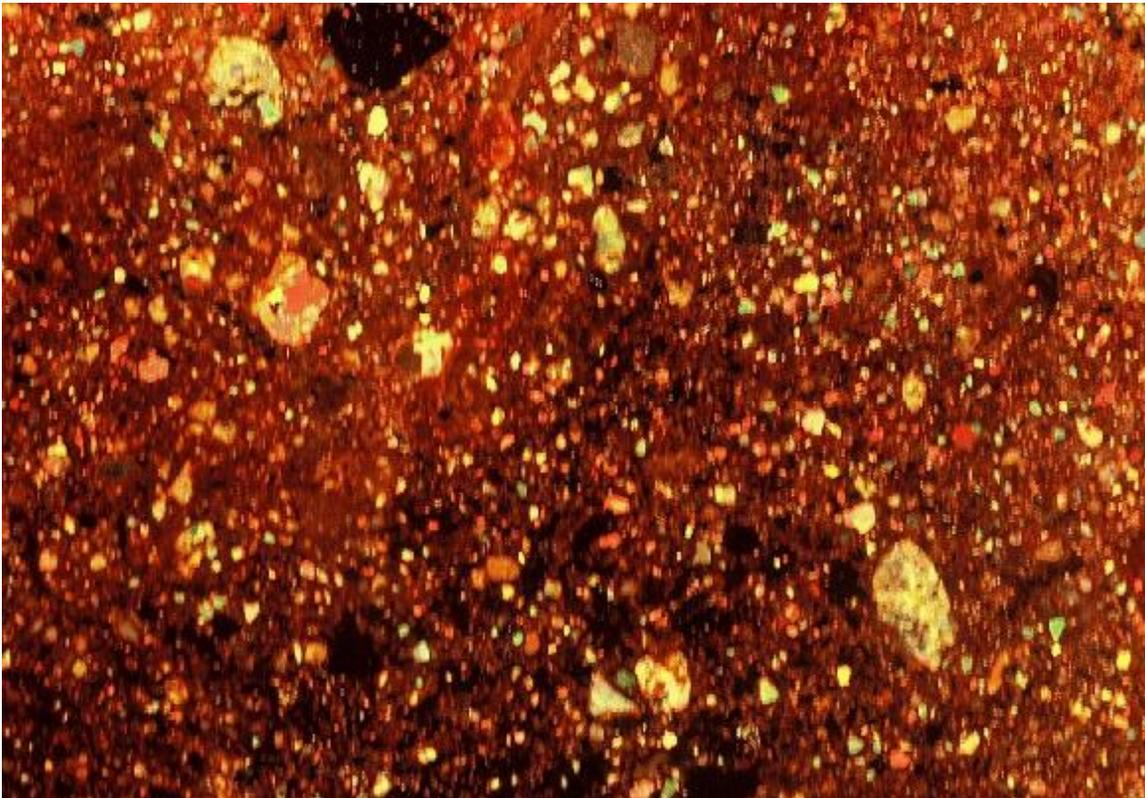
**Cecil clay subsoil compacted by grading activities is dense and has few macro pores. Water ponds over the compacted clay horizon, quickly backs up to the surface, and produces more surface runoff and more frequently.**
