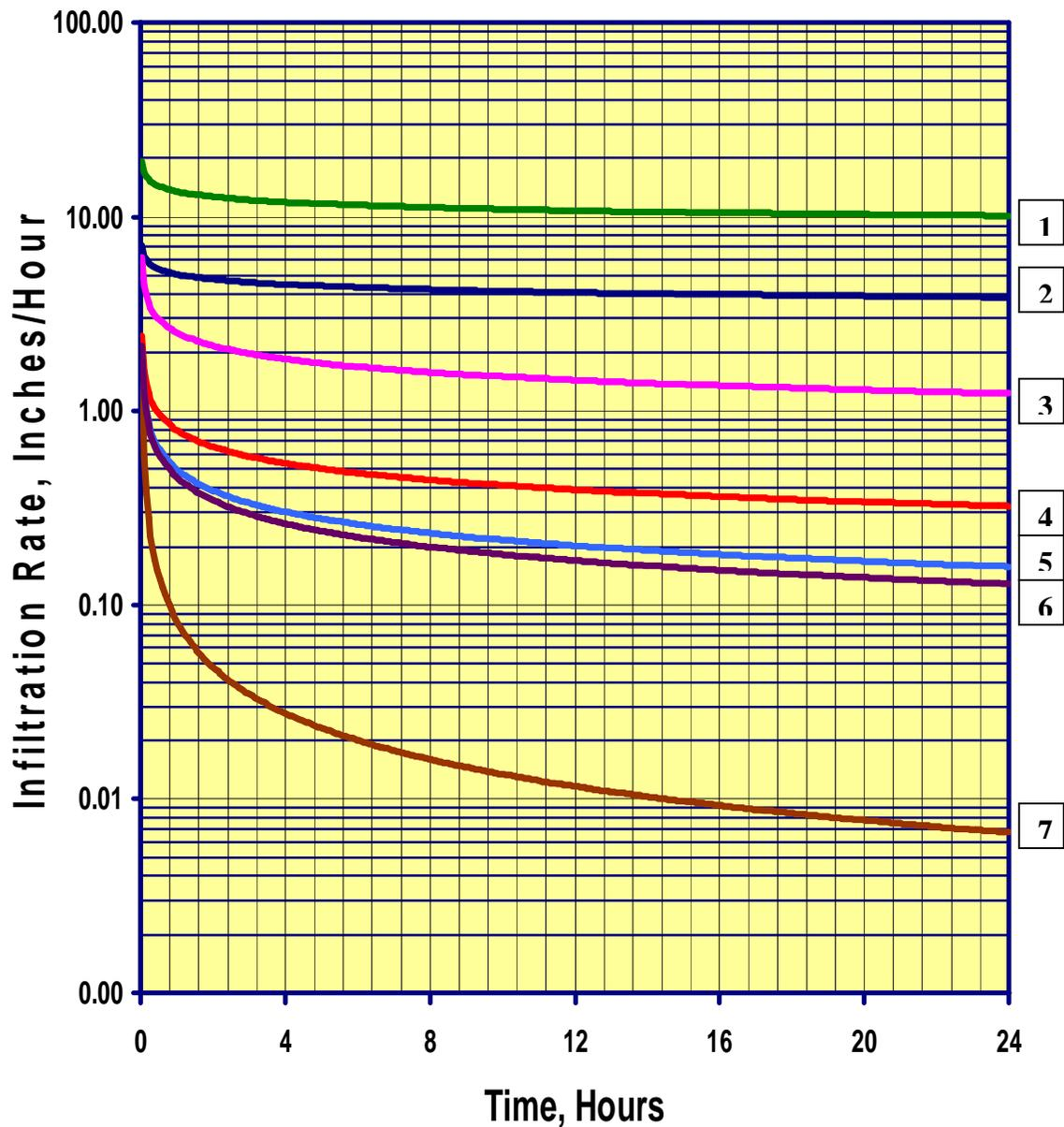
Infiltration rates for Charlotte, NC study for longer storm events. Infiltration rates are shown for storm durations extending out to 24 hours. Curve numbers correspond to numbers and descriptions in Table 2.
