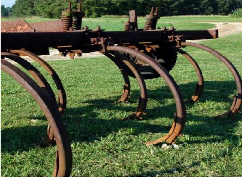
**Agricultural chisel plow used for ripping subsoil to depths from 8 to 12 inches.**
