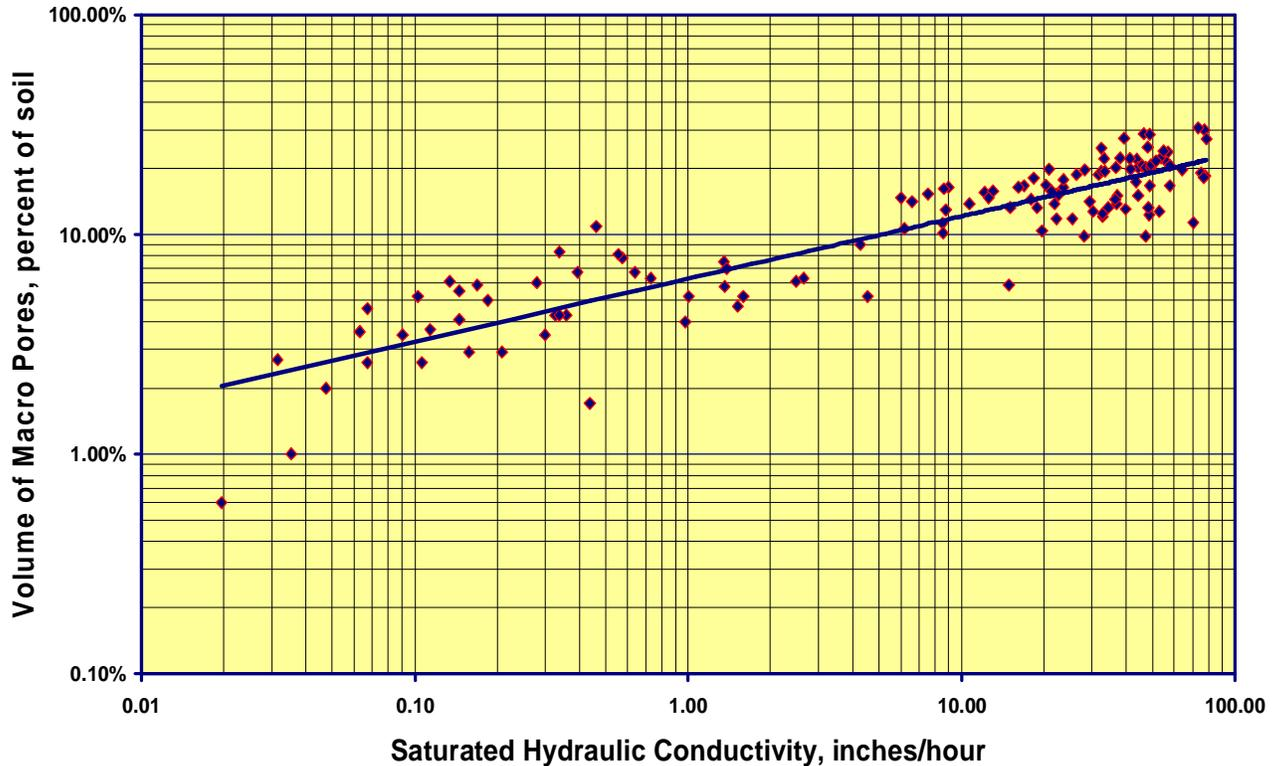
Water flows faster through a soil which has a greater volume of macro pores. Conversely, as the volume of macro pores is reduced the saturated hydraulic conductivity is severely restricted.
